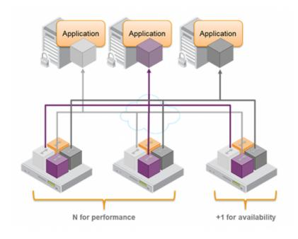
As performance needs grow beyond the performance capacity of three HSMs, it often makes sense to define a second independent group of application servers and HSMs to further isolate applications from any single point of failure. This has the added advantage of facilitating the distribution of HSM and application sets in different data centers.
